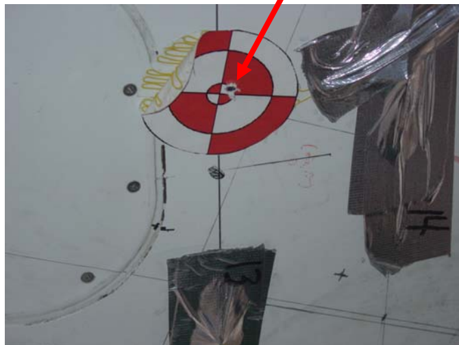
Instrumentation and entrance hole on bottom of wing.
