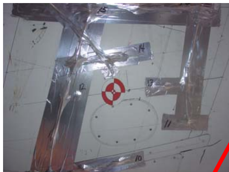
Instrumentation and entrance hole on bottom of wing.
