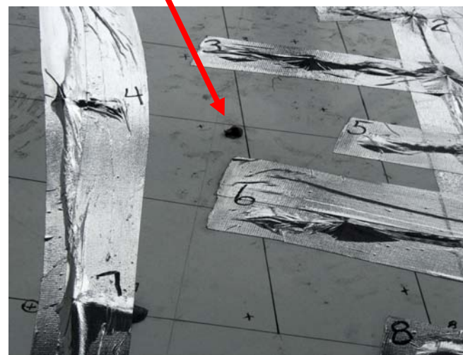
Instrumentation and exit hole on top of wing.
