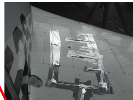
Instrumentation and exit hole on top of wing.
